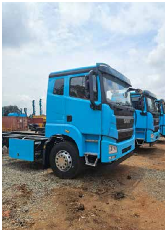
The electric trucks have a range of 170km to 400km, depending on the type of vehicle, the load it is carrying and the terrain.
