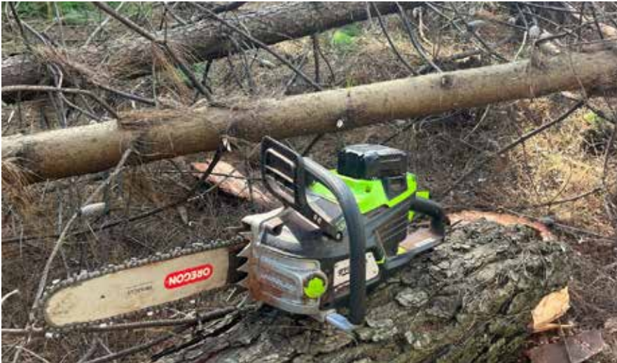
The Greenworks 82V, 5kW HOG chainsaw is powered by batteries that are charged through solar power.
