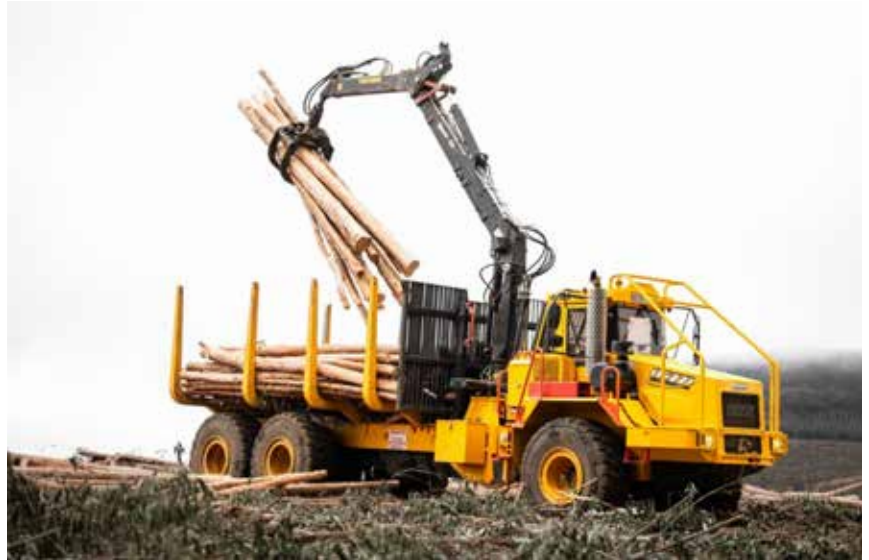
The Dezzi range of Articulated Timber Trucks are designed to fulfill the dual purpose operations of infield loading (up to 25% slope) and short-haul to depot. This allows customers to utilise one self-loading machine, with a single operator, as opposed to three machines with three operators to fulfill the same operation. The Dezzi Articulated Timber Trucks are available in 20-tonne and 30-tonne models.
